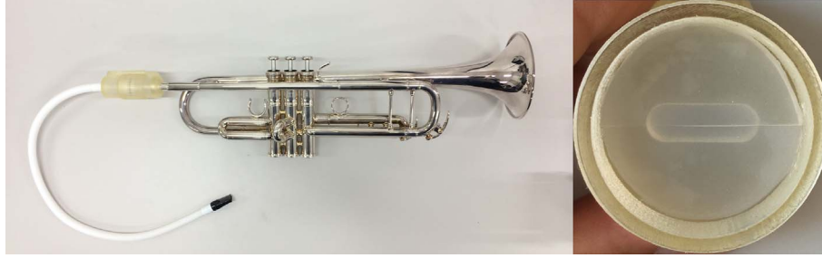
Figure 2. (Color online) A 3D printed version of the pocket artificial buzzing system mounted on a B♭ trumpet, a keyboard-harmonica flexible pipe allows the user to control the pressure in the mouth cavity (left). Front view of the artificial lips mounted on the teeth plate of the mouth unit, with quasi null lip spacing at rest (right).
