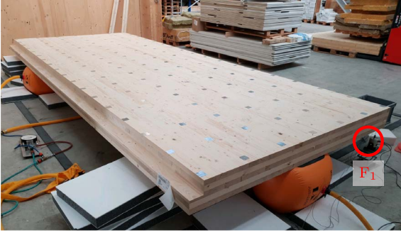
Figure 1. Photo of the experimental set-up for plate CLT200b with shaker located at the F_1 excitation point.
