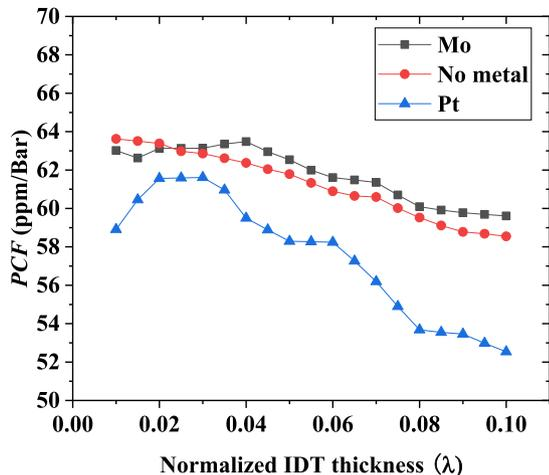
**Figure 5.** PCF for the different metal layer materials as a function of normalized IDT thickness.
