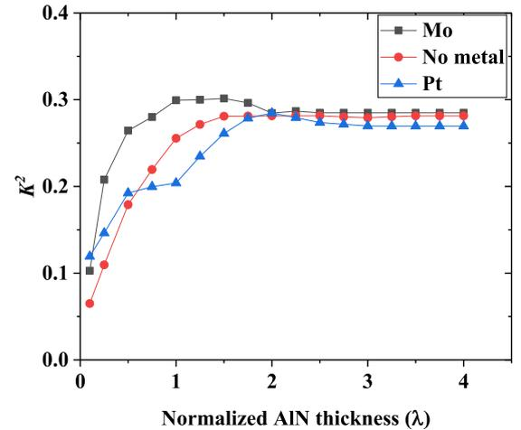
**Figure 4.**  $K^2$  for the different metal layer materials as a function of normalized AlN thickness.
