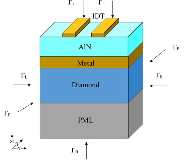
**Figure 1.** Quasi-3D periodic FEM model used in the simulation (not to scale).
