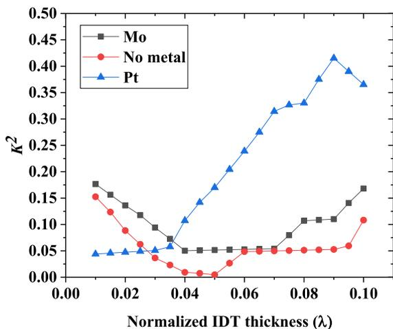
**Figure 6.**  $K^2$  for the different metal layer materials as a function of normalized IDT thickness.
