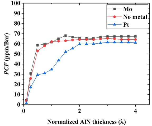
**Figure 3.** PCF for the different metal layer materials as a function of normalized AlN thickness.
