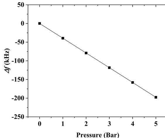
**Figure 7.** Dependence of  $\Delta f$  on pressure.
