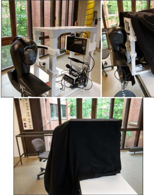
**Figure 2.** MASAVE with simulated subject without textile cover (top left), with textile covering the MASAVE structure (top right), and with textile covering the MASAVE and the entire torso to block out light (bottom).
