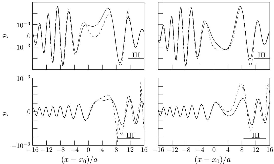
**Figure 5.** Acoustic potential above and below source; left-hand column: real part; right-hand column: imaginary part; solid line: numerical; dashed line: approximation. Top row: field above source and plate; bottom row: field below source and plate.
