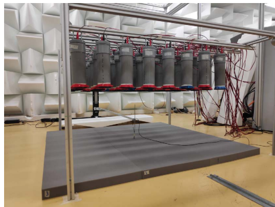
Figure 2. Picture showing the experimental setup, the 64-loudspeaker array being positioned above a layer of polyurethane foam.
