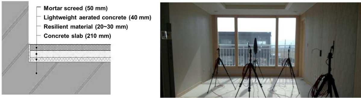
Figure 2. Floor section composition in typical Korean apartment buildings (left) and field measurement setup in accordance with KS and Korean building regulations (right).
