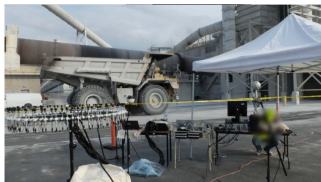
Figure 1. Sound environment capture in an open-air lime mine using a double-layer circular microphone array. Recordings were performed near a mine crusher (left) and with trucks passing at few meters from the array (right), among others.
