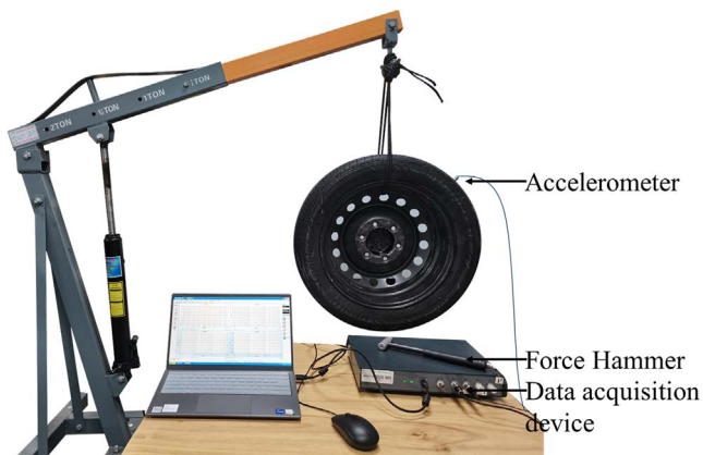
Figure 3. Tire modal test environment.
