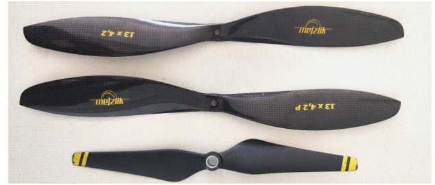
Figure 6. From the top: (i) Mejlzik 13'' \times 4.2 propeller counter-clockwise used at rear position, (ii) Mejlzik 13'' \times 4.2 clockwise propeller used at front position, and (iii) DJI 9450 propeller.
