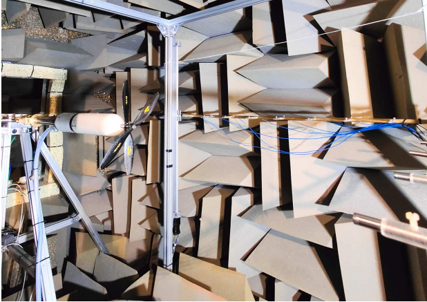
Figure 2. Fairing, cooling hose, supporting stand, and microphone setup in the anechoic room ALCOVES.
