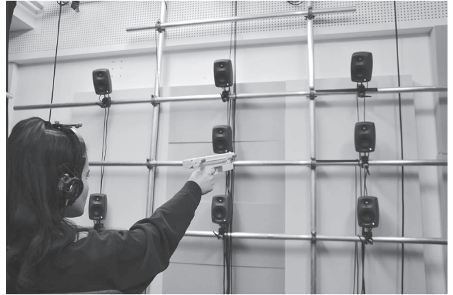
Figure 1. Participant wearing circumaural open headphones during the experiment task in a studio room ( RT_{30} = 0.2 s). Motion-tracking is enabled via an OptiTrack system (NaturalPoint Inc.) with markers attached to the headphones and the toy gun.
