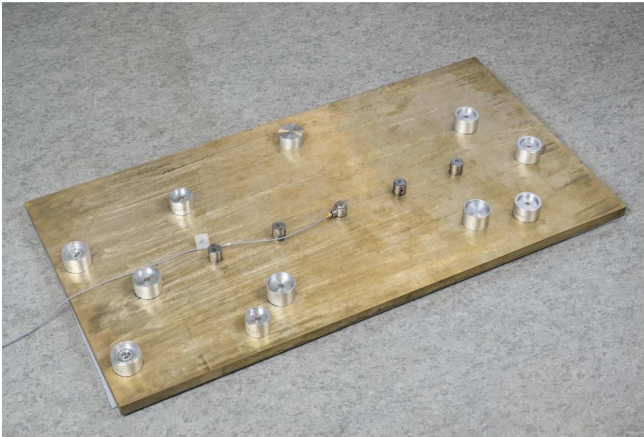
Figure 5. Receiving plate with force sensor.
