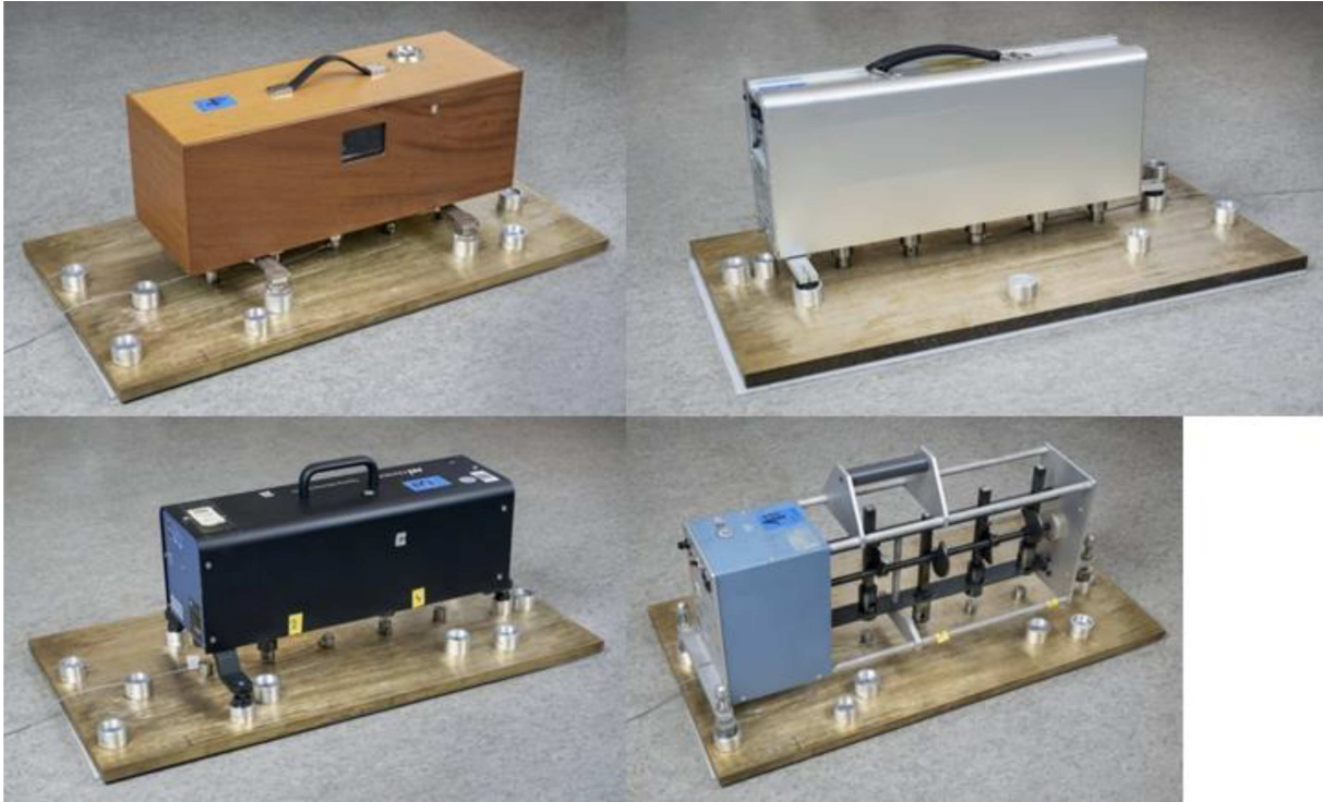
Figure 6. Different types of tapping machines positioned on the receiving plate.
