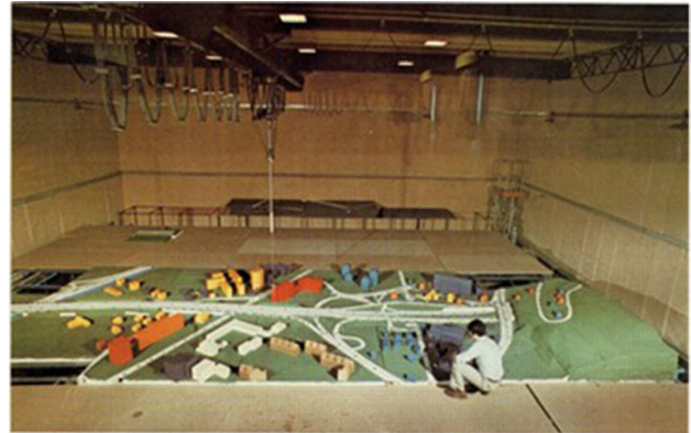
Figure 7. The “Maquette” laboratory for environmental noise evaluations in 1/100 scale models.
