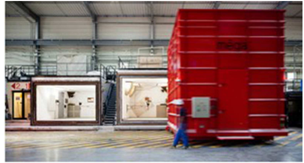
Figure 16. CSTB Acoustic test laboratory (LABE); moving (therefore slightly blurred) room in red; fixed rooms behind.
