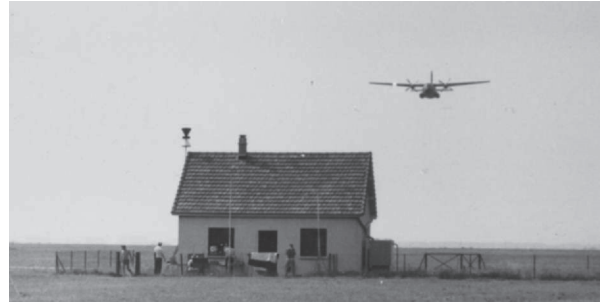
Figure 4. Experimental house, subjected to supersonic flyover events.
