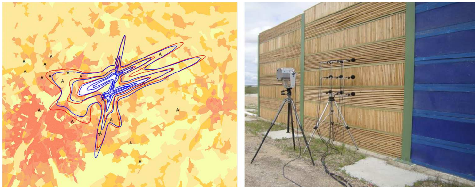
Figure 4. Example of calculated noise contours around Brussels Airport (left) and “Quesst method” measurement set-up determining the sound absorption of noise barrier during a round robin test.
