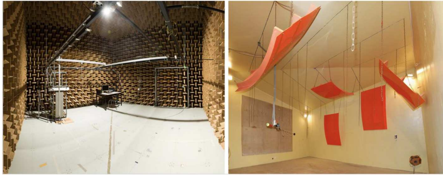
Figure 3. View into the anechoic (left) and reverberant (right) room.
