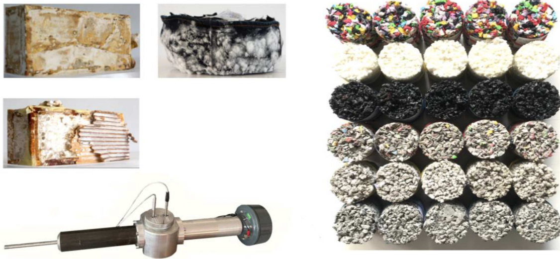
Figure 7. Recently investigated materials for sound absorption in the framework of the EU-MSCA doctoral network ActaRe-Build (top left: biomaterial mycelium, right composites based on recycled plastics, bottom left: impedance tube used for the characterization) [61].
