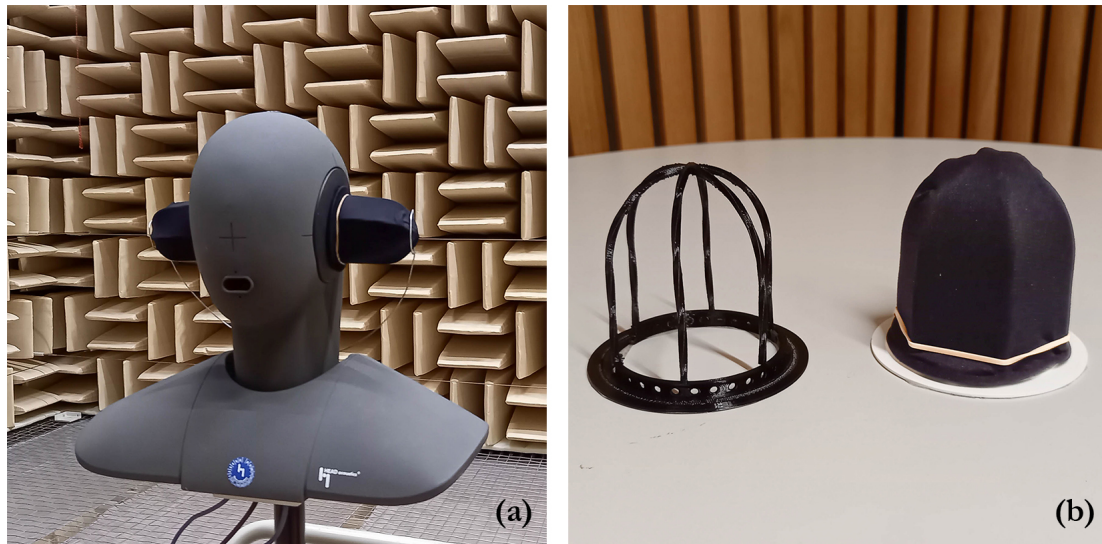
Figure 2. (a) Dummy head with mounted windshields on both ears. (b) The windshield's plastic grid (left) covered with nylon fabric (right).
