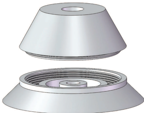
Figure 3. Schematic diagram of the connection between the radiating head and the front cover in practical applications.
