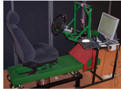
Figure 14. Test bench for the evaluation of vibration discomfort [81].
