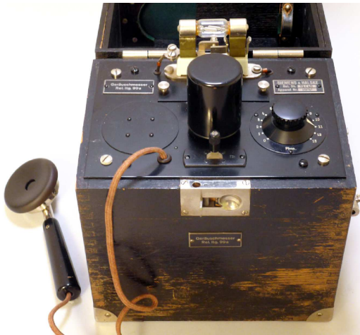
Figure 4. Loudness meter from Barkhausen, produced by Siemens & Halske starting 1927. Photograph of the device in the HAPS collection of TU Dresden [11], no. 15–1.
