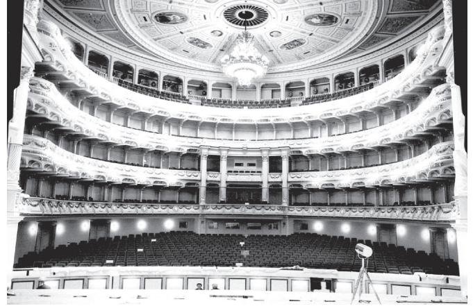
Figure 11. Auditorium of the Semper opera Dresden during acoustic testing in 1984 with marked measuring places and a directional loudspeaker on the stage. Photograph by Rolf Dietzel, reproduced from [30].
