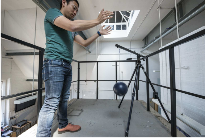
Figure 3. ISO rubber ball drop used for experimental validation of prediction models on impact sound insulation.
