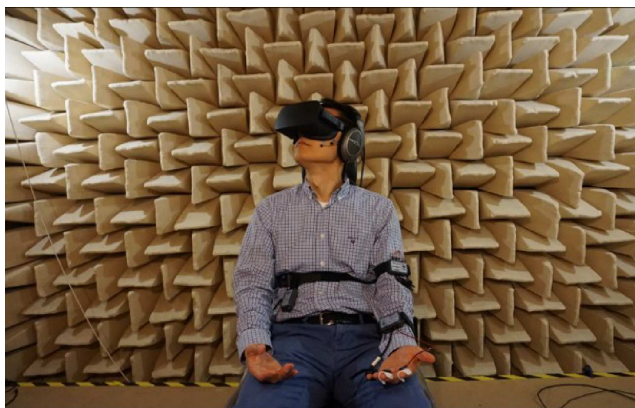
Figure 5. A participant engaged in a VR experiment, wearing electrodes to measure physiological responses to soundscapes.
