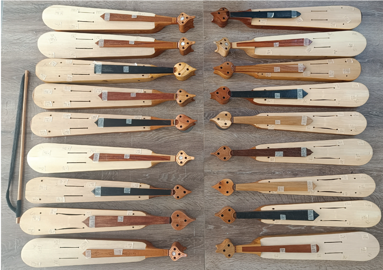
Figure 1. The 18 Karadeniz kemenche samples analysed in this study, displaying regional variations in size, body proportions, and construction characteristics representative of Eastern Black Sea craftsmanship traditions (The strings and related components have been disassembled for experimental modal analysis).
