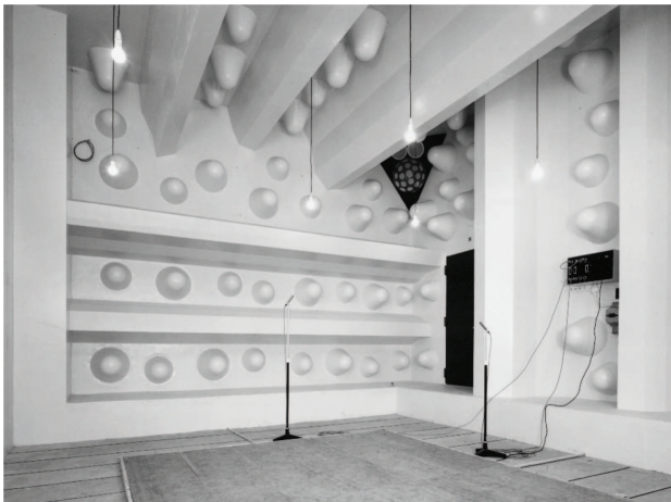
Figure 11. One of the reverberation rooms built 1963, 240 m 3 .
