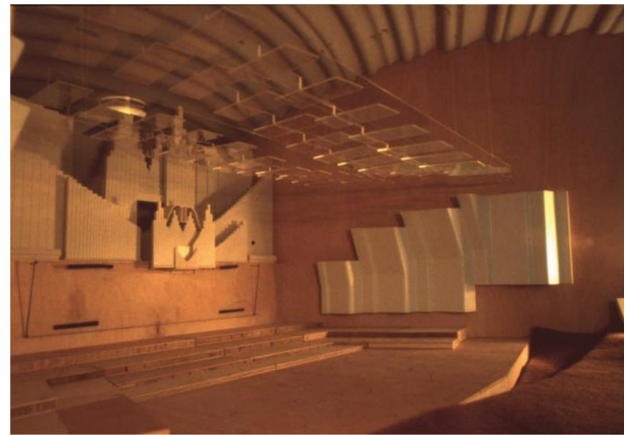
Figure 14. Scale model 1:20 used for investigations on the old DR concert hall, 1988. Wall reflectors and a suspended reflector array were part of the refurbishment.
