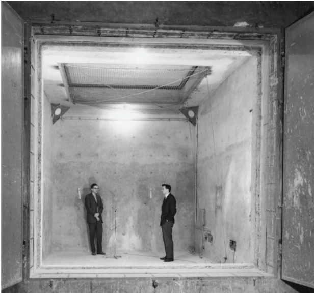
Figure 4. Reverberation chamber, built around 1935–40, 96 m 3 . The two persons are Ole Juhl Pedersen (left) and Jørgen Kristensen (right).
