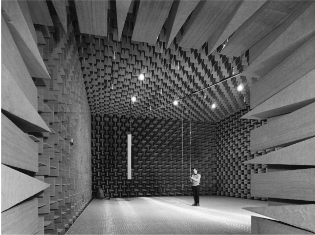
Figure 10. The anechoic room built 1963, 1000 m 3 free volume. The person is Peter Koefoed Møller.
