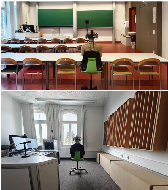
Figure 3. Rooms under investigation. Top: A HATS positioned at the listening position in the room under investigation, which is the congruent playback room in the experiment. Bottom: A HATS positioned in a recording studio, which is the divergent playback room in the experiment. During the experiments, the virtual room model shown in Figure 4 was presented through the HMD in both rooms.
