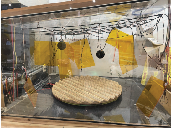
Figure 8. Small-scale reverberation chamber in Sydney, Australia.
