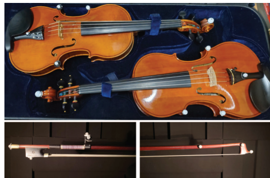
Figure 1. Markers placed at different points on the violins and the bow.
