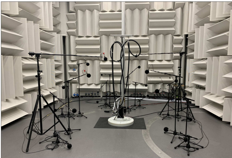
Figure 5. Test setup in a hemi-anechoic chamber and the compressor test bench in an adjacent room.
