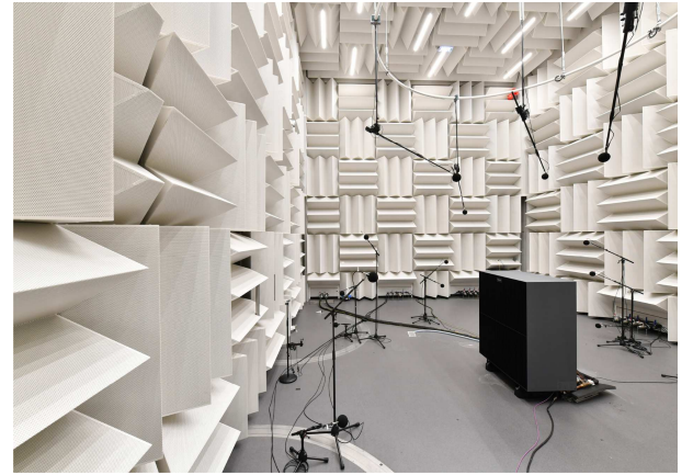
Figure 9. Acoustic development of the air-to-water heat pump demonstrator in a hemi-anechoic chamber.
